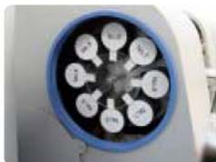
Motorized 8 hollow cathode lamp turret accessory
