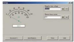
Obtain reliable and accurate results by using the Energy control feature to manually optimize atomiser position and setup, Use the Auto-balance feature to ensure energy level, and optical alignments are optimized when using background correction.
